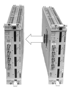
Figure 2-10: Connecting the logic analyzer modules together
