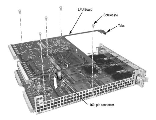
Figure 6-8: LPU board removal
