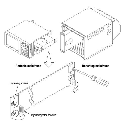
For more detailed information on installing modules, refer to *Appendix D: TLA700 Module Installation* in the *Tektronix Logic Analyzer Family User Manual*.
