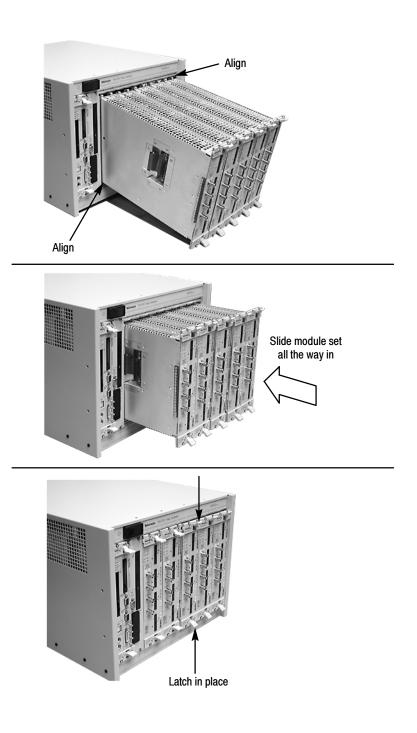
Figure 2-11: Installing the merged module set in the mainframe
