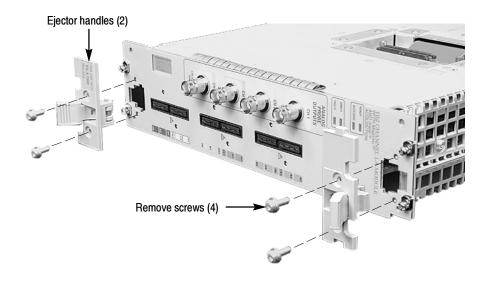
Figure 6-3: Injector/ejector handle replacement
