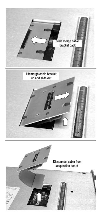
Figure 6-11: Removing the merge cable assembly
