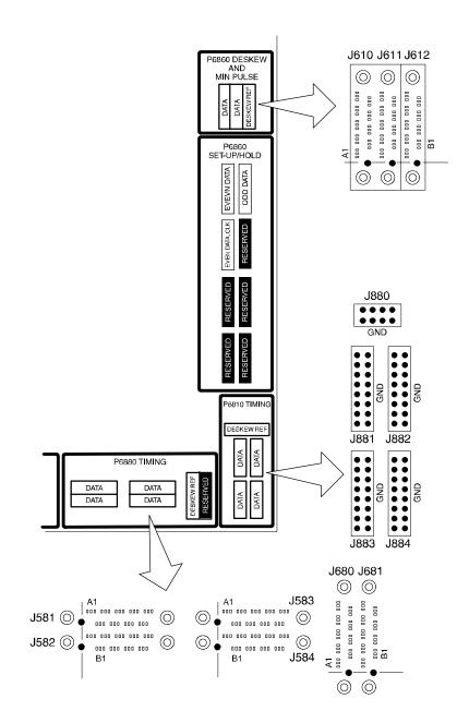
Figure 5-4: Deskew procedure probe connections
