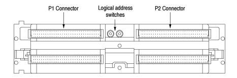
Figure 2-7: Rear panel controls and connectors
