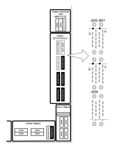
Figure 4-6: P6860 Setup & Hold procedure connections
