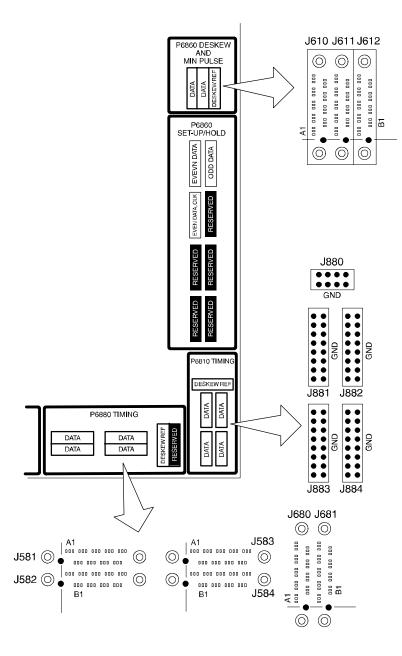
Figure 4-5: Module+Probe timing procedure probe connections
