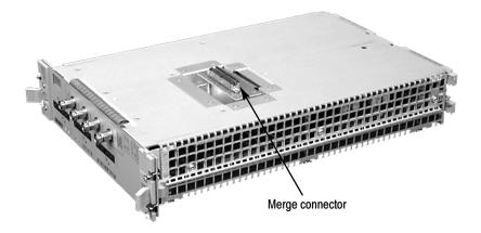
Figure 2-6: Merge connector (shown in the extended position)
