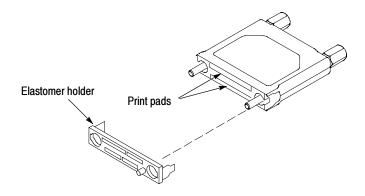
Figure 6-1: Cleaning the probe heads
