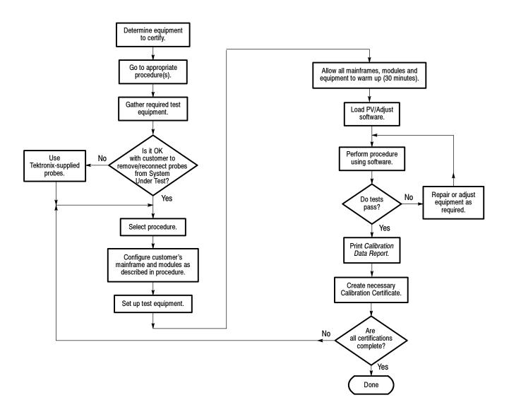
Figure 4-1: Calibration/certification procedure flow chart
