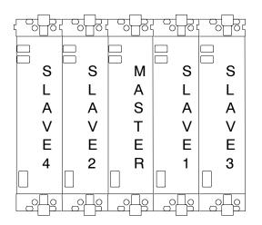
Figure 1-1: Location of modules in merged configurations
