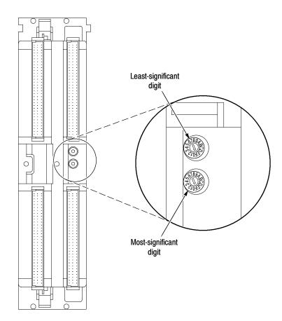
Figure 2-1: Logical address switches
