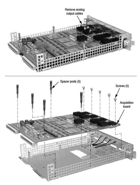
Figure 6-12: Removing the acquisition board from the chassis
