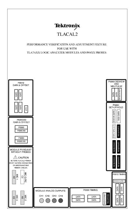
Figure 4-3: TLACAL2 test fixture connections
