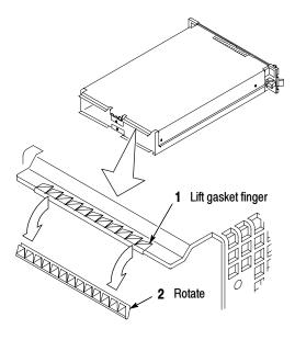
Figure 6-13: Rear EMI gasket removal
