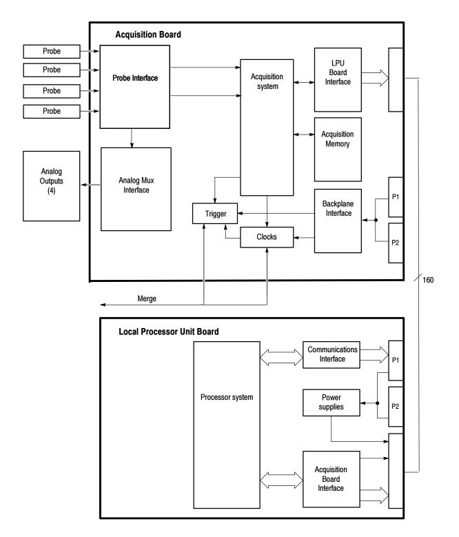
Figure 9-1: Logic analyzer block diagram
