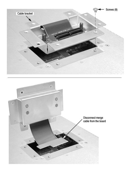
Figure 6-4: Removing the merge cable bracket from the cover
