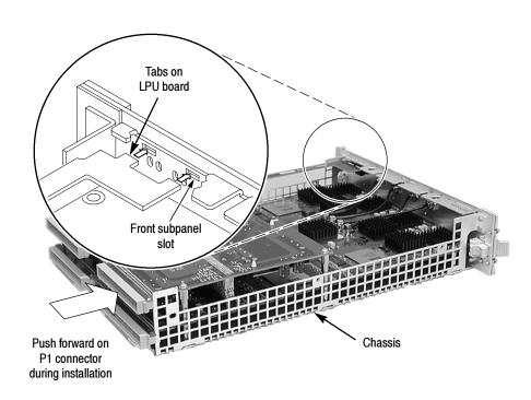
Figure 6-9: Inserting LPU board tabs into front subpanel
