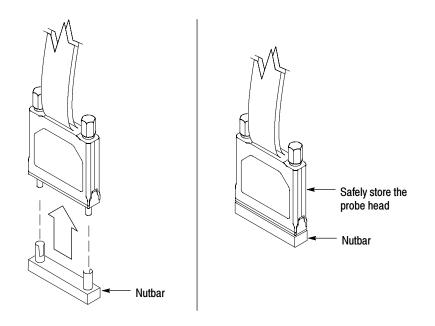
Figure 6-2: Storing the probe head
